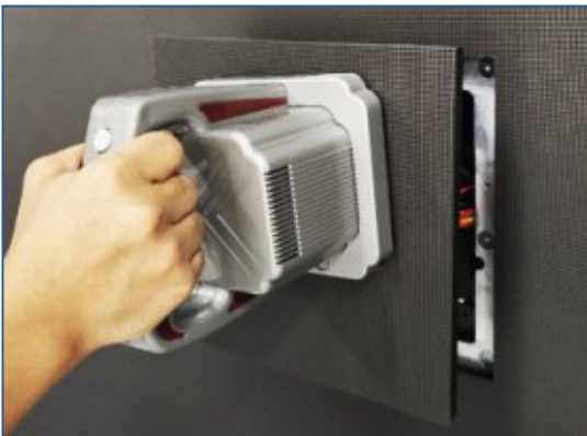
Step 3: Gently pull the tool, the module will be separated from the cabinet.
