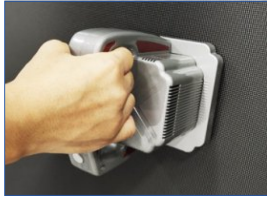
Step 2: Put the front maintenance to contact the module, and make sure that the module is roughly in the center.
