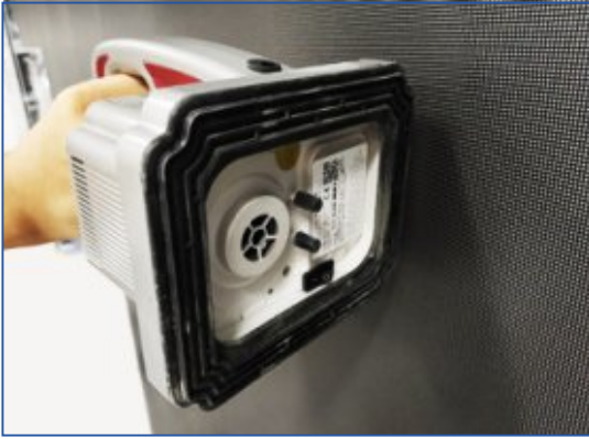
Step 1: Stand the front maintenance tool sideways near the cabinet.
