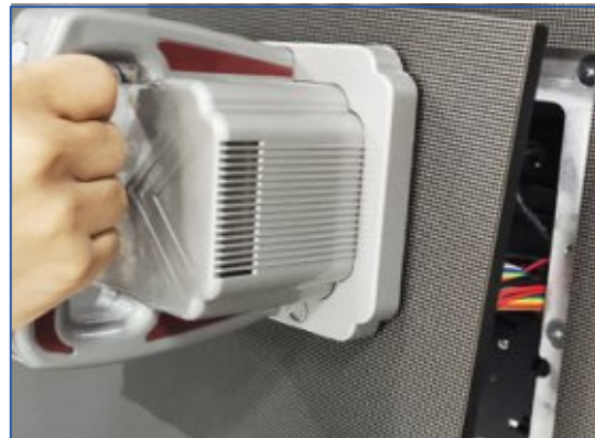
Step 4: Install the replaced module through the tool and install it in the same way.
